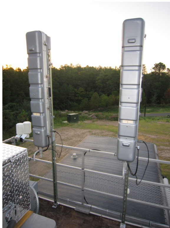
Figure 3-2. Denuder/filter pack samplers.
