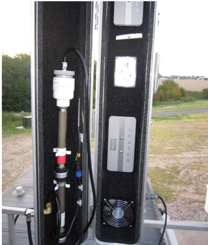
Figure 3-3. Installed denuder/filter pack sampling train.
