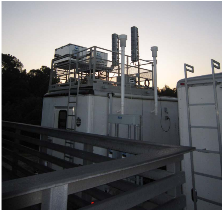
Figure 3-1. Sampling trailer with denuder/filter pack samplers.
