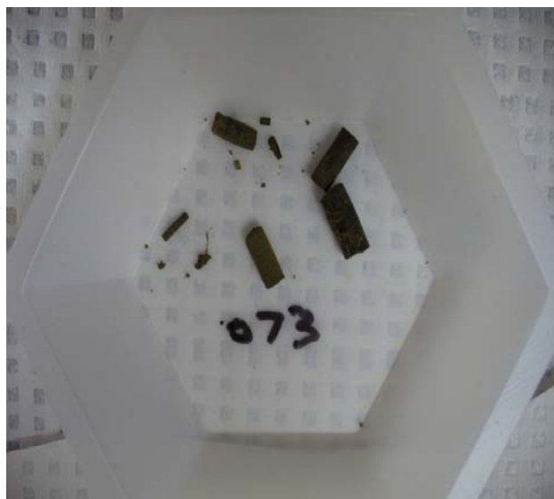
Figure 2-16 Propellant Removed from Soil Sample 1885-02-SS-073
