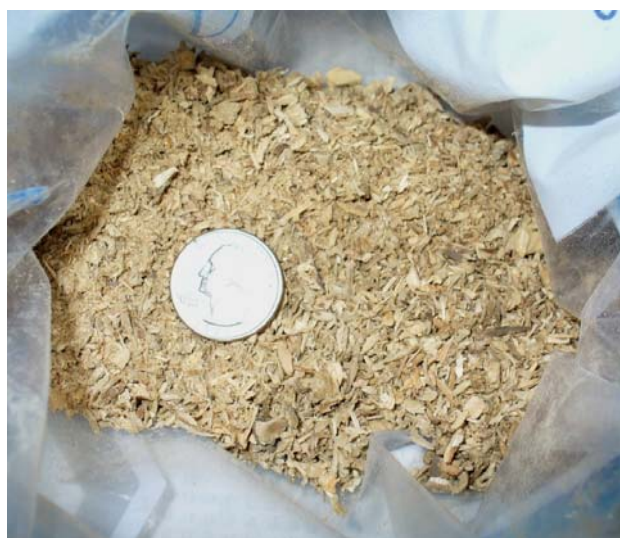
Figure 2-12 Blender Homogenized Wood Less Than 1/4 inch
