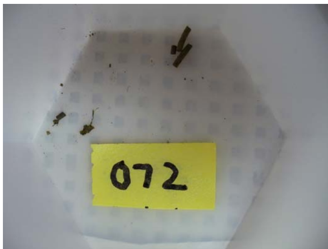
Figure 2-17 Propellant Recovered from Soil Sample 1885-02-SS-072
