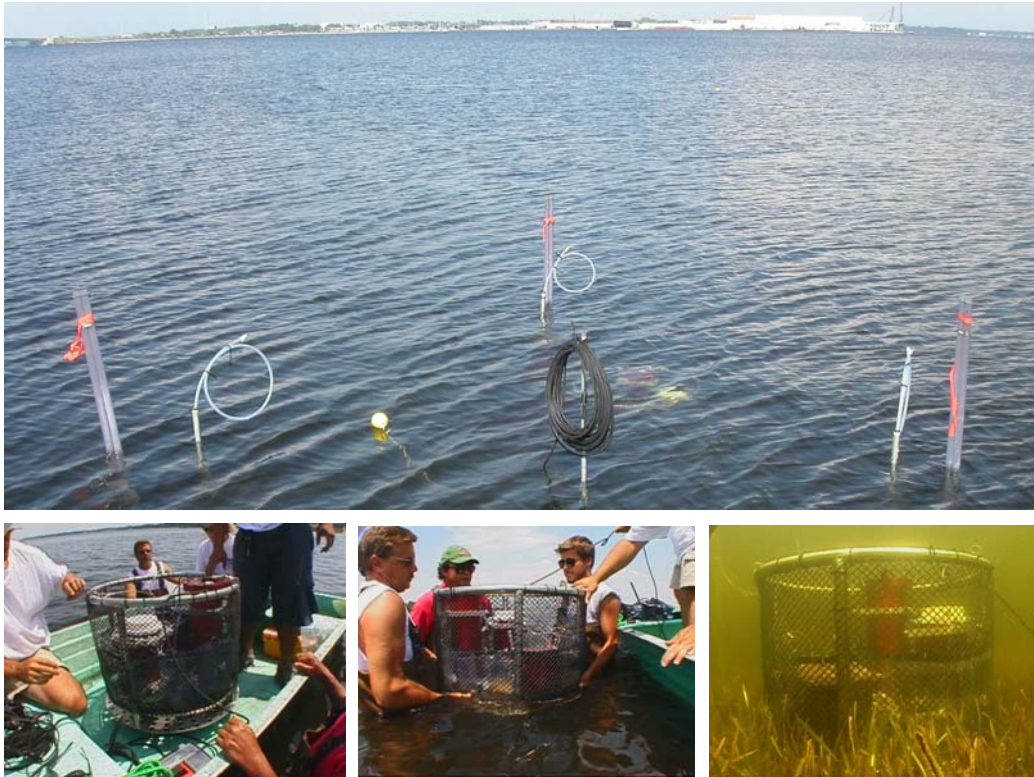
Figure 12. The UltraSeep Being Deployed in St. Andrews Bay (bottom left and center); Installed on the Bottom (bottom right); and Viewed from Above, Including the Array of VOC and Level-Logging Piezometers at Station T4-4 (top).
