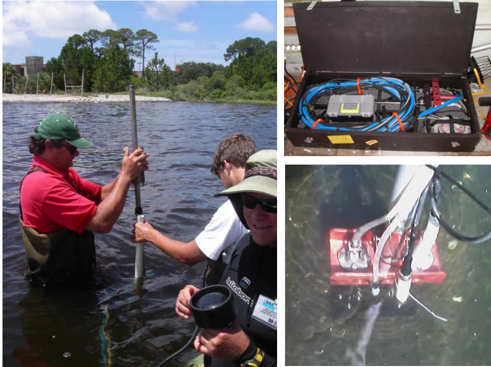
Figure 5. Deployment of the Trident Probe in St. Andrews Bay.
