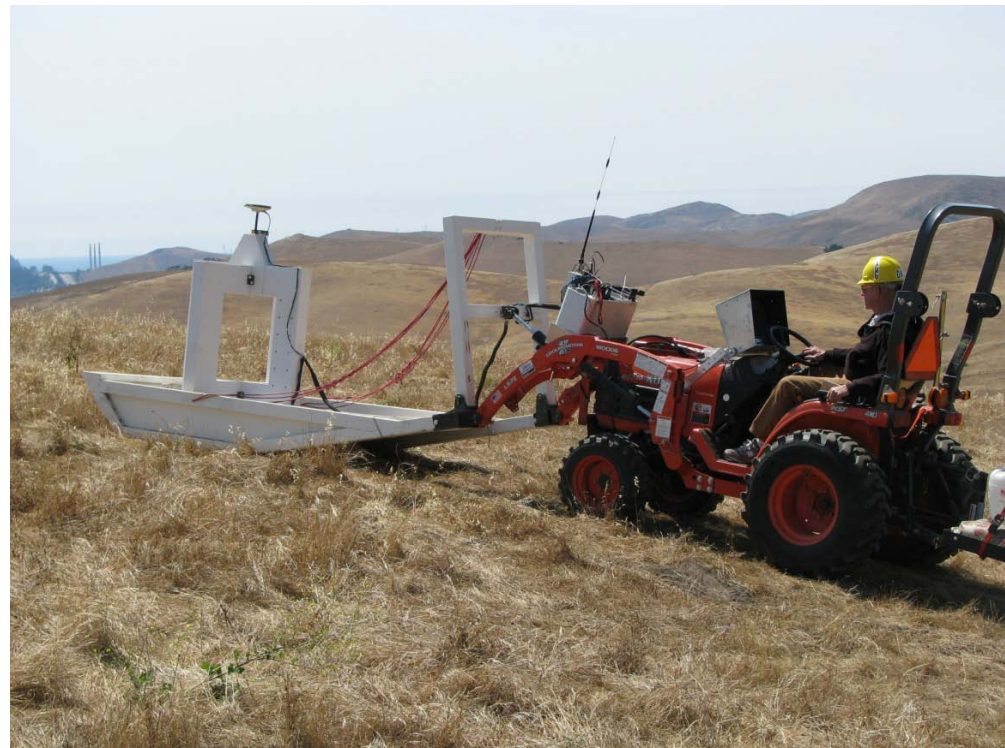
Figure 1. Photos showing the MM antenna array together with the electronics package and control console (inset above).
