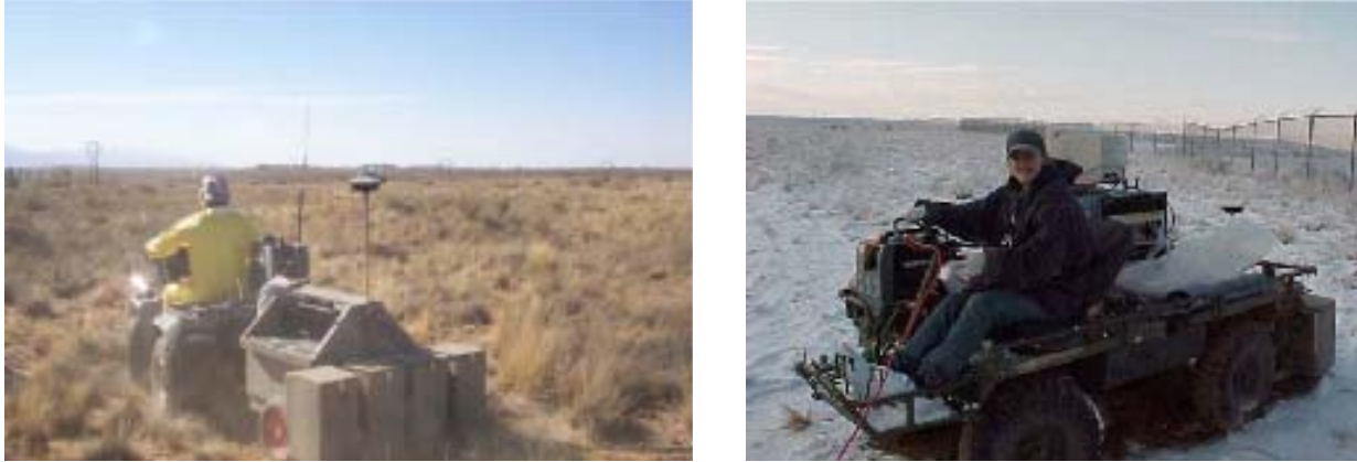
Figure G-1. Mobile data acquisition system configurations
