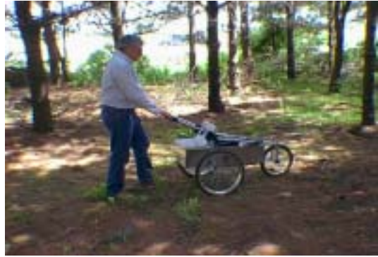
Figure 2-3. Radiation scanning system
