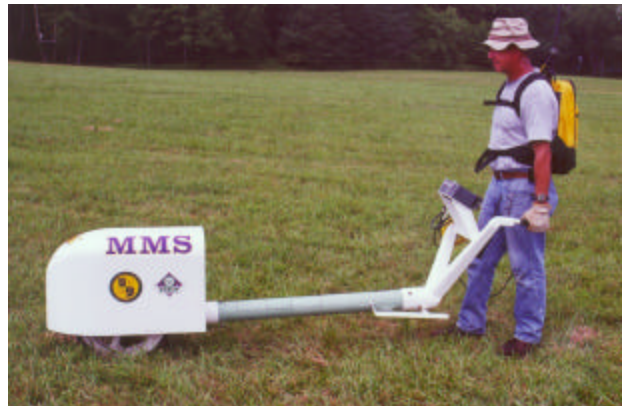
Figure 9. MMS Deployed with Protective Hood and GPS Navigation Hardware.
