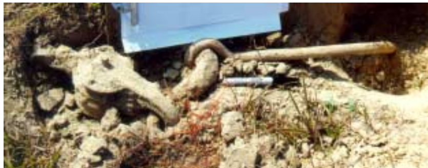
Figure 5. Example of Non-Ordnance Remediated at L Range. (This item is part of a block and tackle used for guy-cables for a test tower.)
