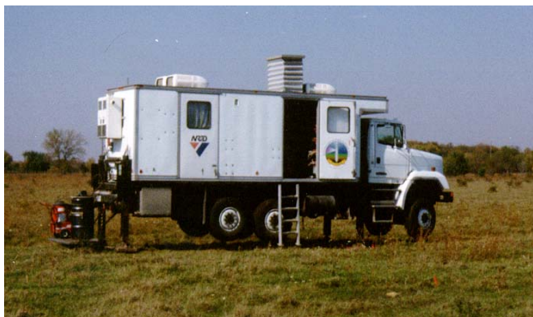
Figure 4. Photograph of Navy Cone Penetrometer Test (CPT) Vehicle.
