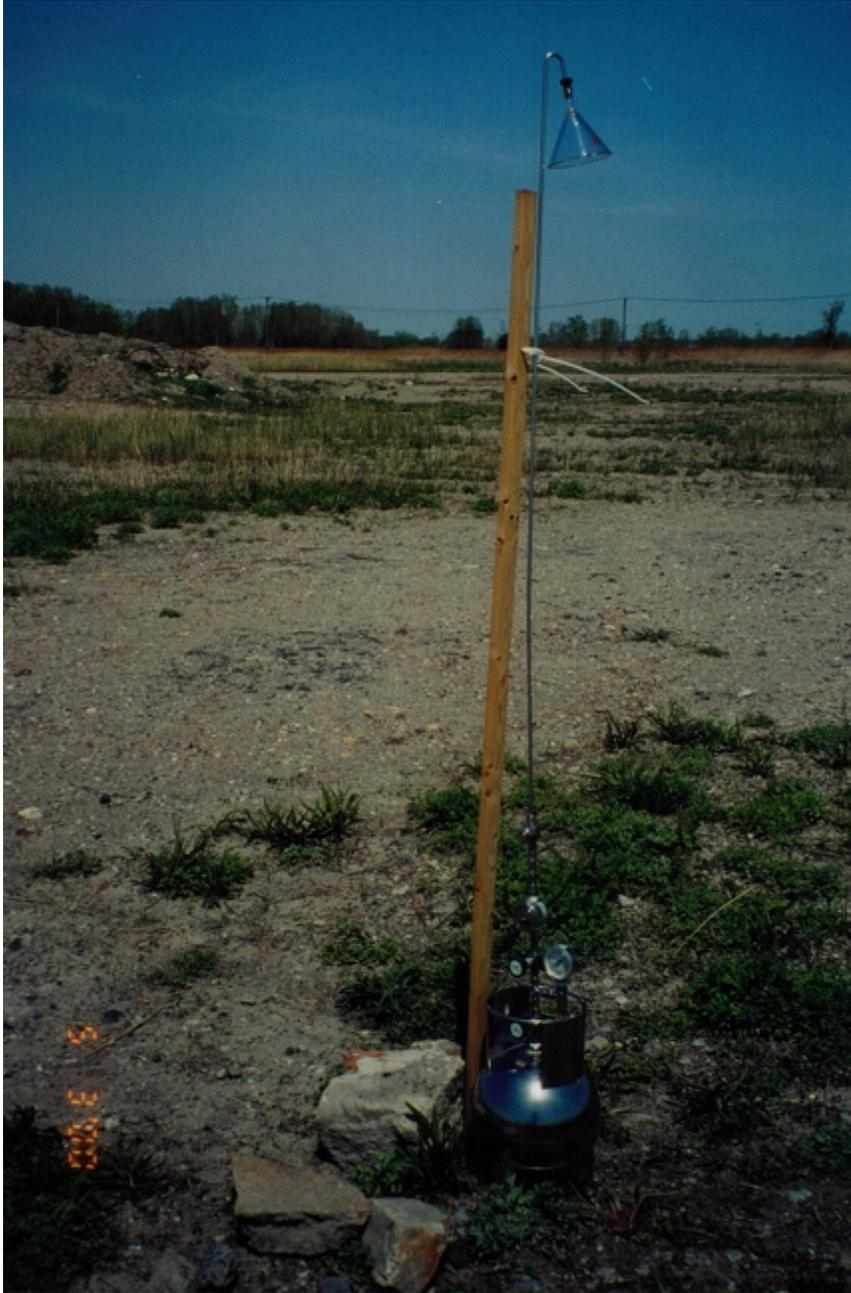
Figure 6. VOC Canister Sample.
