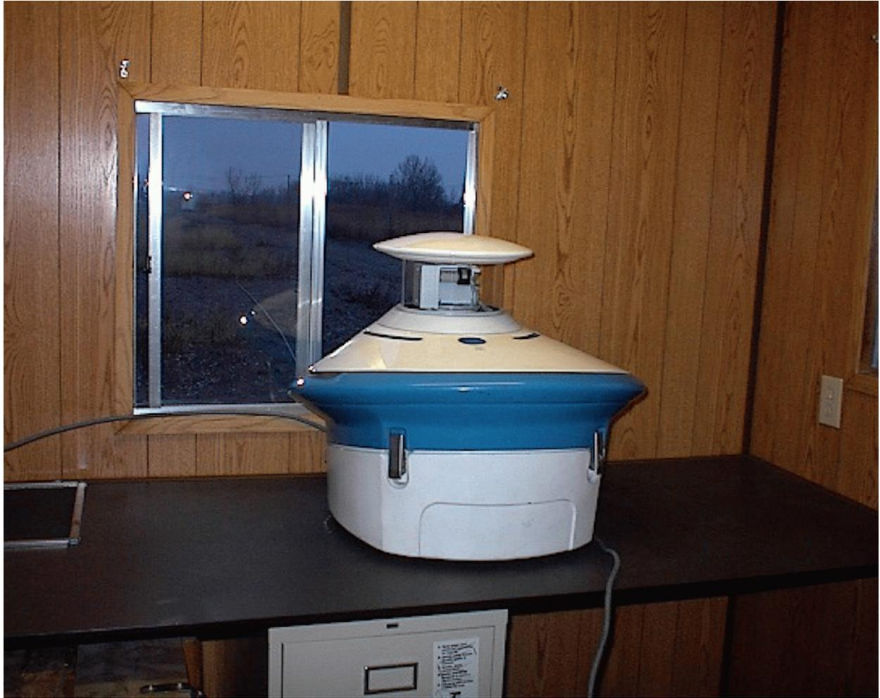
Figure 2. UV-DOAS Receiver inside Trailer #1.
