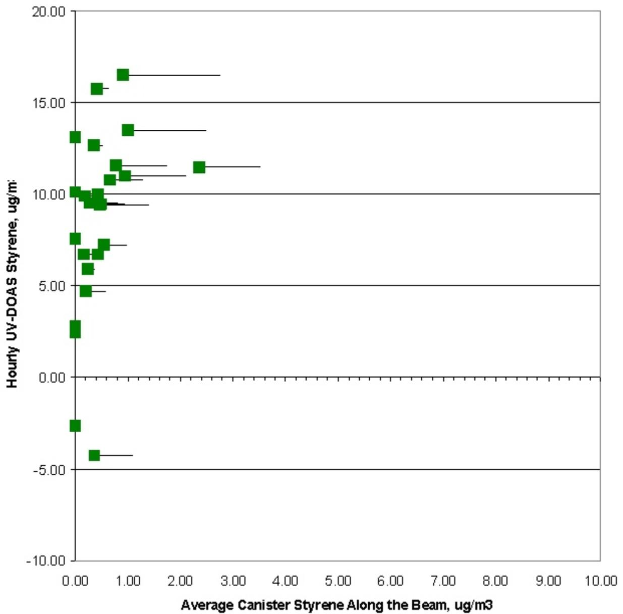
Figure 25. Effect of canister styrene variation vs. UV-DOAS.
