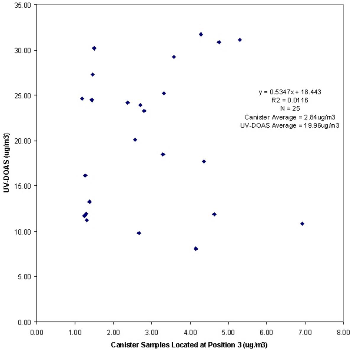
Figure 17C. Benzene concentrations: UV-DOAS data versus data obtained from canisters located in Position 3.
