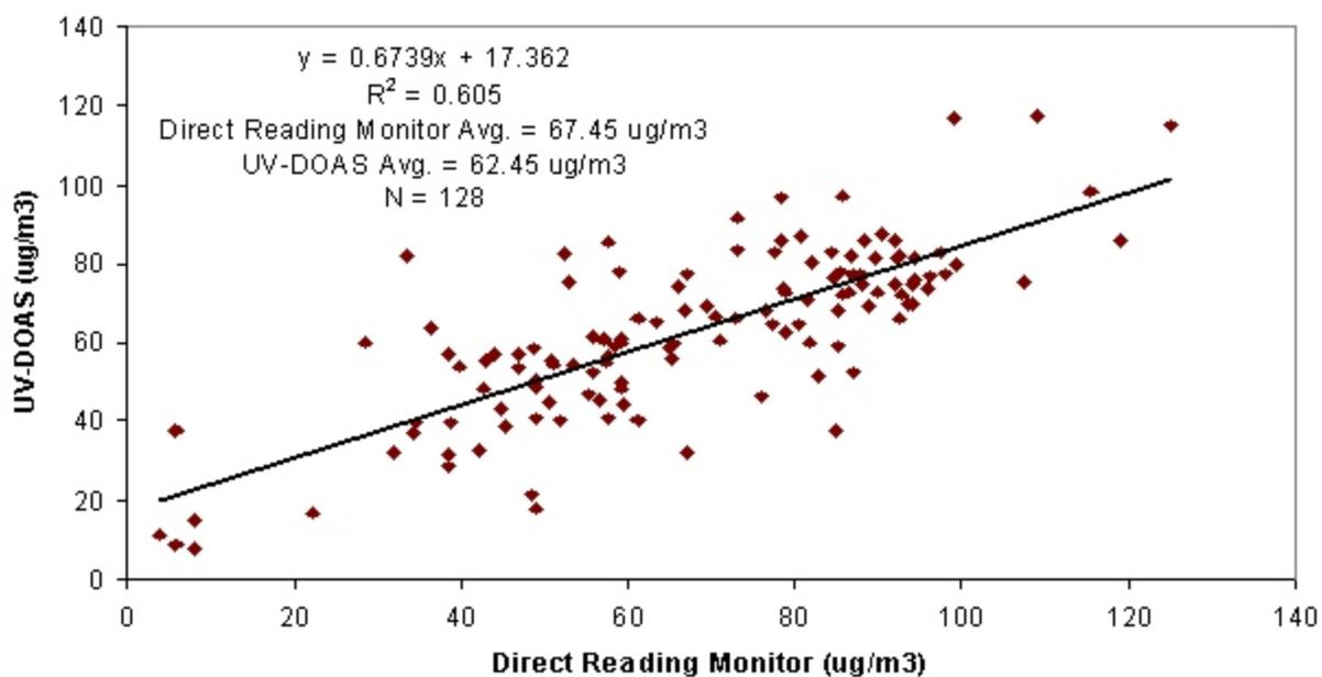
Figure 10. Direct reading and UV-DOAS ozone concentrations, (A) nighttime, 1900 to 0500 hours, (B) daytime, 0600 to 1800 hours.
