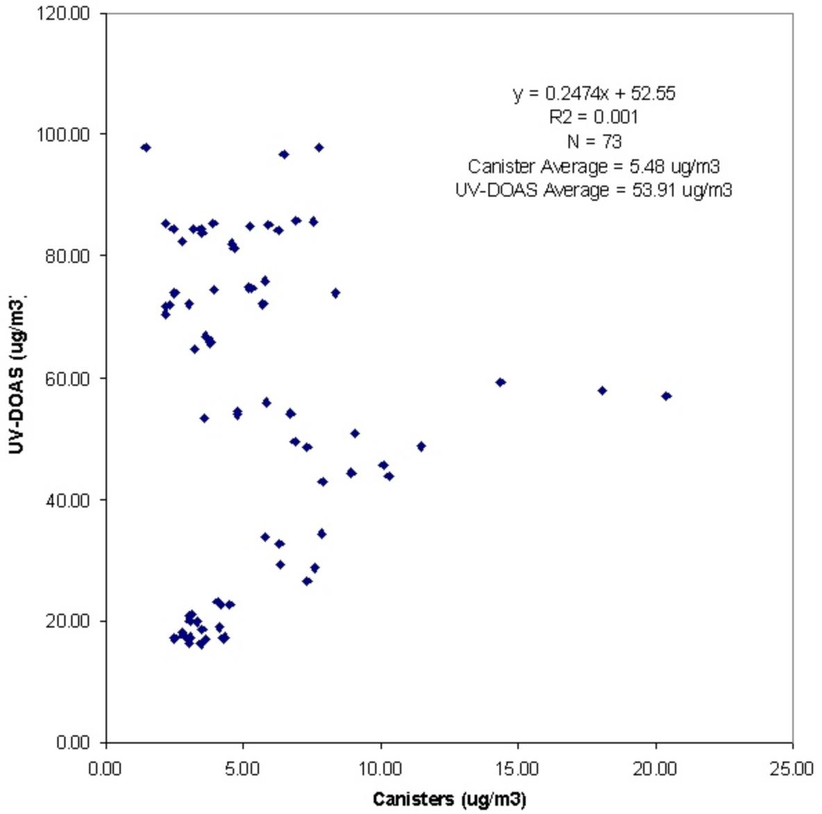
Figure 29. Relationship plot of the sum of benzene, toluene, and m-xylene concentrations obtained by the UV-DOAS and canister samples.
