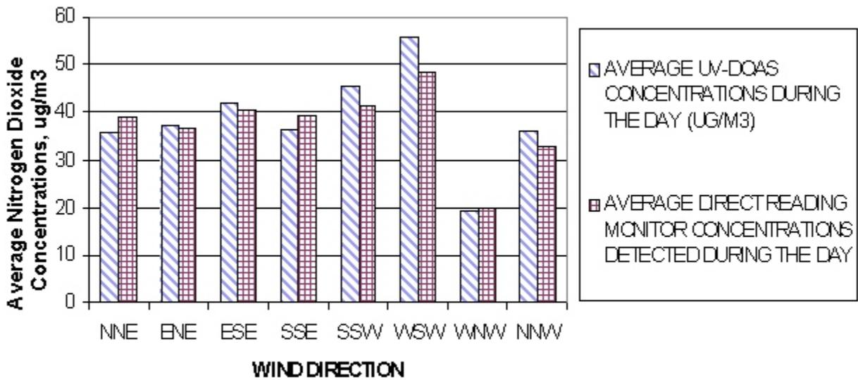
Figure 11. Average NO<sub>2</sub> concentrations vs. wind direction, (A) nighttime, 1900 to 0500 hours (B) daytime, 0600 to 1800 hours.
