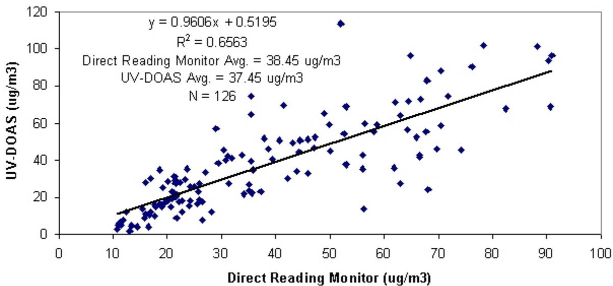
Figure 9. Direct reading and UV-DOAS nitrogen dioxide concentrations (A) nighttime, 1900 to 0500 hours, (B) daytime, 0600 to 1800 hours.
