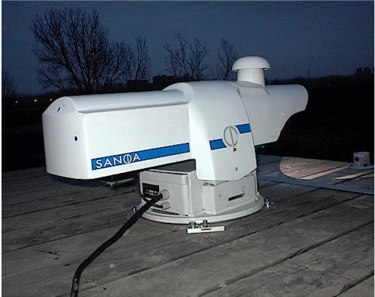
Figure 1. UV-DOAS Projector on the roof of Trailer #2.
