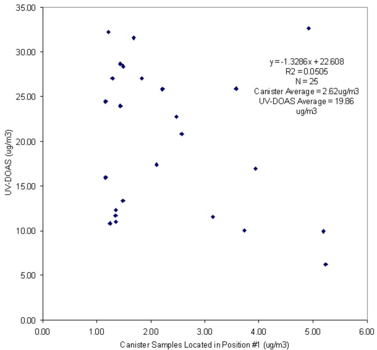
Figure 17A. Benzene concentrations: UV-DOAS data versus data obtained from canisters located in Position 1.
