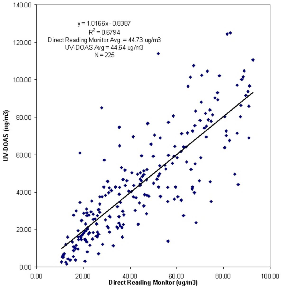
Figure 8. Comparison of direct reading and UV-DOAS nitrogen dioxide concentrations.
