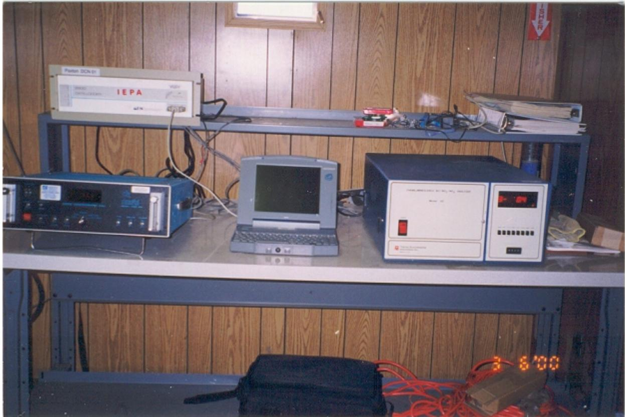
Figure 5. TECO 42 NO<sub>x</sub> Monitor (on the right) and Dasibi Model 1003AH Ozone Monitor (on the left) inside Trailer # 2.
