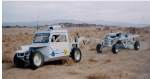
**Figure 1. The *MTADS* deployed with the magnetic sensor array**
