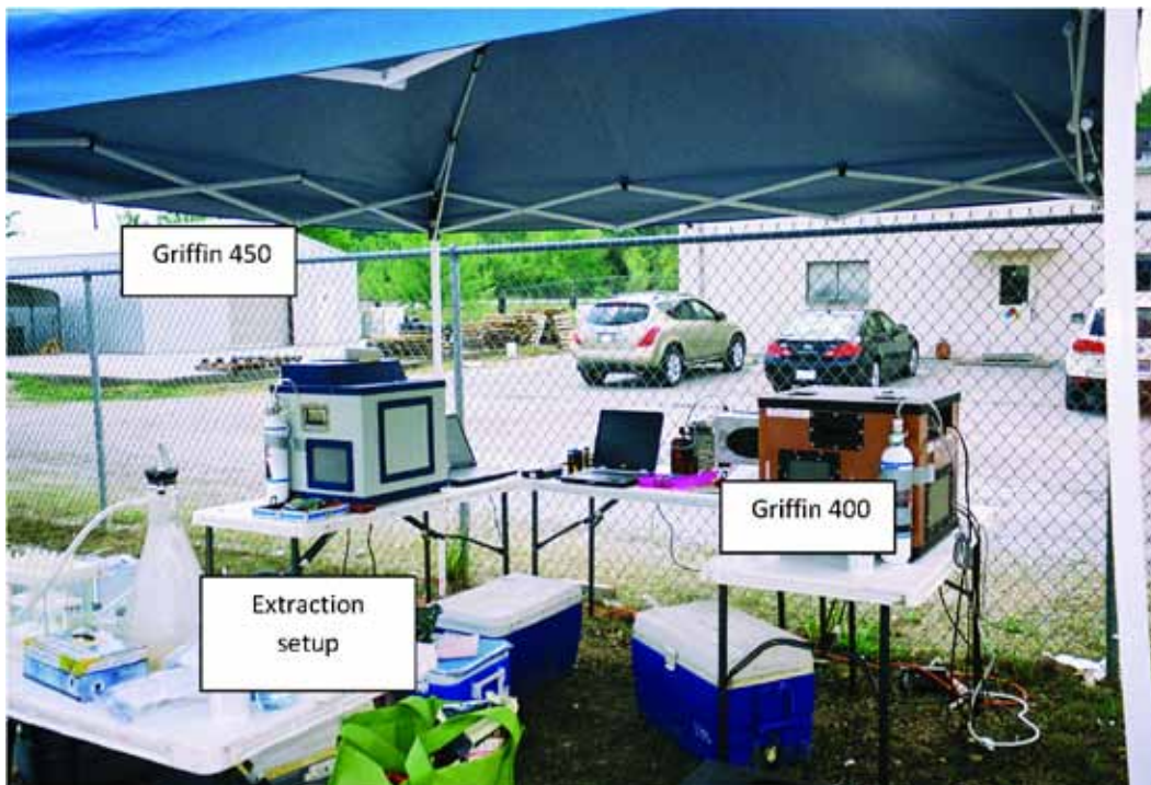
Figure 2.2. Field setup for the Griffin 400 (right) and 450 (left); extraction setup is shown in the front left.
