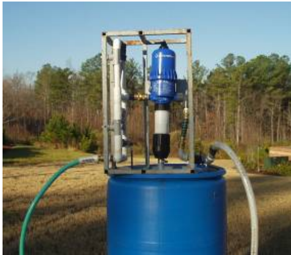
Figure 5.8 Setup of Automatic Metering System for Dilution of Concentrated Emulsion Product (Photo courtesy of EOS Remediation, Inc.)
