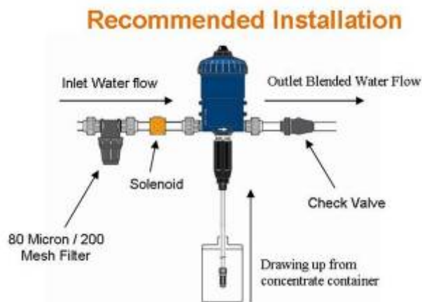
Figure 5.8 Setup of Automatic Metering System for Dilution of Concentrated Emulsion Product (Photo courtesy of EOS Remediation, Inc.)
