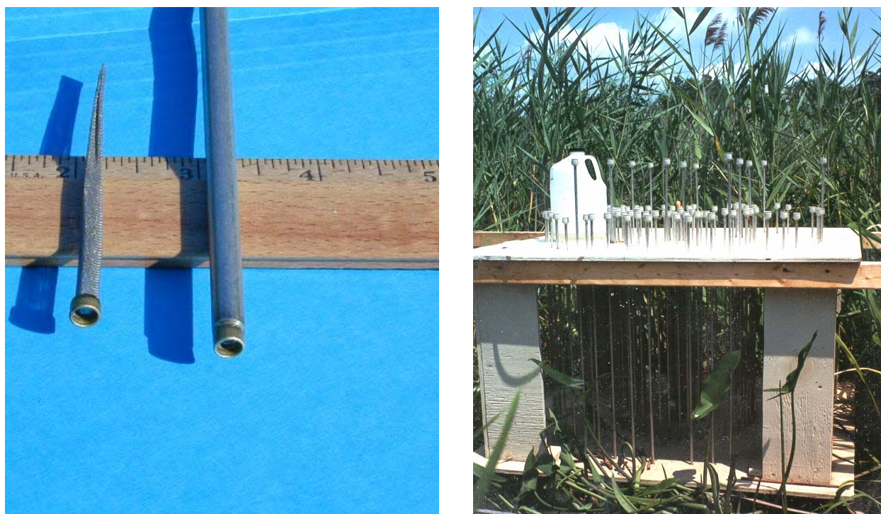
Figure 20. Photographs of tubing and screen components of tubing sampler (left) and the tubing sampler array at wetland field site (right). USGS photos
