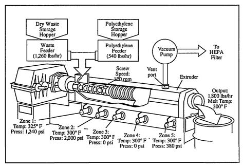
Polyethylene Encapsulation System
