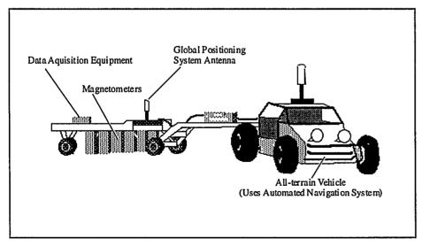
Magnetometer Towed Array
