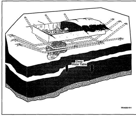
Horizontal/Directional Drilling Concept
