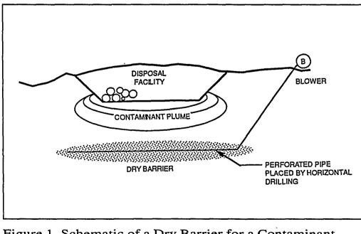
a subsurface application, the injection and extraction wells would be placed using either horizontaldrilling technology (shown) or systems of vertical wells.
