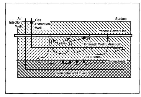
Schematic Diagram of Horizontal Well In Situ Air Stripping
