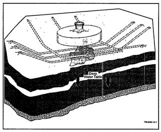
Horizontal Wells Beneath A Buried Tank
