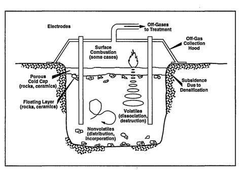
Disposition of Materials During ISV Processing
