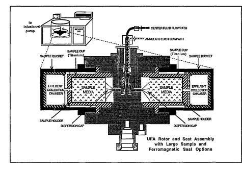
hydraulic conductivity on about 50 samples were measured in less than 6 months using one UFA<sup>™</sup>instrument. The data were used to extend the understanding of subsurface interactions under actual field conditions at Hanford Site for characterization, remediation, and predictive modeling. The database could not have been developed without using the UFA<sup>™</sup> method.
