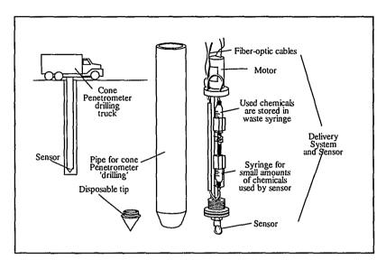
Figure 1. Light Transmission Optrode
