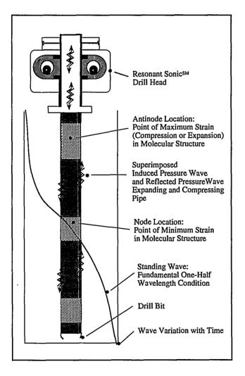
Figure 1. ResonantSonic<sup>™</sup> Energy
