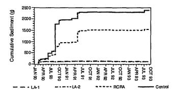
Figure 6. Cumulative sediment from the Landfill Capping Demonstration plots as a function of time for all cap designs at Hill AFB.
