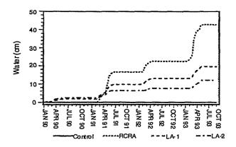
Figure 3. Cumulative barrier lateral flow as a function of time for all cap designs at Hill AFB.
