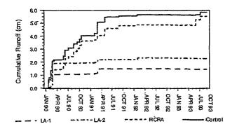
Figure 5. Cumulative runoff from the Landfill Capping Demonstration plots as a function of time for all cap designs at Hill AFB.
