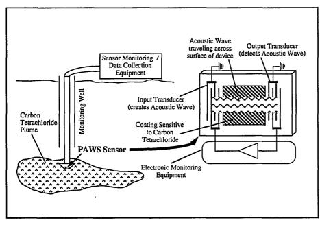
Schematic of a Portable Acoustic Wave Sensor
