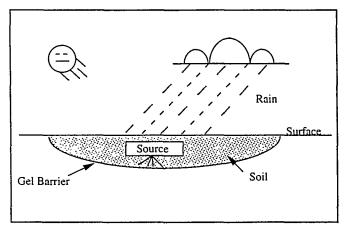
Figure 1. Gel Barrier for In Situ Use.
