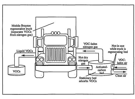
Decoupled Brayton-Cycle Solvent-Recovery Heat Pump for Small Emitters
