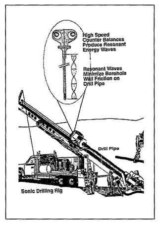
Figure 2. Schematic of ResonantSonic<sup>SM</sup> Drilling
