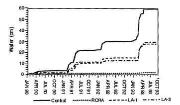
Figure 4. Cumulative leachate flow as a function of time for all cap designs at Hill AFB.
