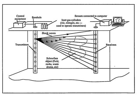
training of personnel in both source operation and operation of winches for fielding tools. The seismic sources are pneumatic and require compressed gas (usually air, argon, or nitrogen) that is supplied from tanks at the surface. The only physical output will be the vented gas. Effects of failure are restricted to high-pressure hazards and are easily controlled. Components must be periodically pressure tested for continued integrity. Electrical power for running direct-current motors
