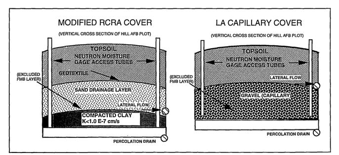
Figure 2. Comparison of EPA-RCRA Cap and the Los Alamos Capillary Cap.
