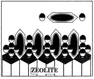
Figure 1. TMA-Zeolite Selective Sorption Mechanism
