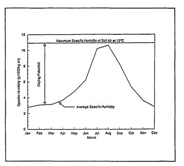
Figure 2. Drying Power of Albuquerque, NM Air Adjusted to 13°C to Reflect Subsurface Drying of Soils.
