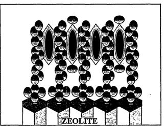
Figure 3. HDTMA-Zeolite Non-Selective BTEX Removal
