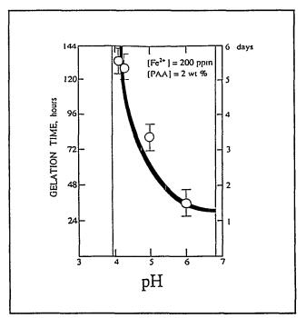
Figure 2. The Effect of pH on Gelation Time.
