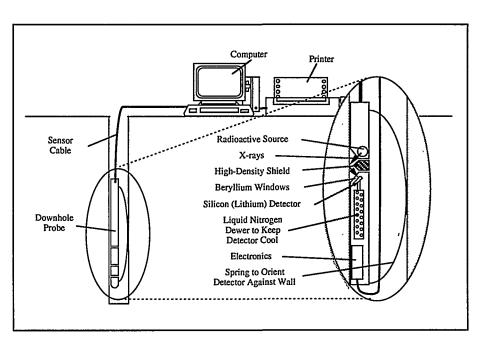
Prototype XRF System
