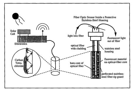
Figure 2. Reversible Fiber-Optic CCl<sub>4</sub> Sensor
