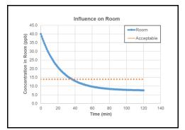
Figure 7. Air treatment unit influence on indoor air concentrations (idealized example after initial startup)
