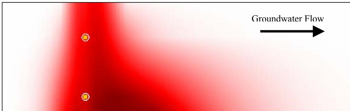
**Figure 5.4** Model simulation of sediment oil distribution in a profile along the direction of groundwater flow, 28 days after emulsion injection.
