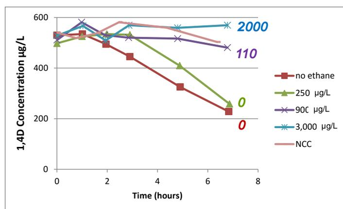
**Figure 5-9.** Biodegradation of 1,4-dioxane by the enrichment culture for a range of initial ethane concentrations. Final ethane concentrations also are shown in the figure. Average of duplicate samples are shown. NCC= no cell control.
