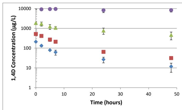
**Figure 5-8.** Biodegradation of 1,4-dioxane by the MBAFB enrichment culture under resting conditions. Experiments with initial 1,4-dioxane concentrations ranging from approximately 10,000 to 200  $\mu\text{g/L}$  are shown. The averages of triplicate samples are shown. Error bars represent 95% confidence intervals. Abiotic controls showed no decreasing trend in 1,4-dioxane concentrations (data not shown).
