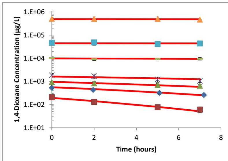
**Figure 5-10.** Model regression to the 1,4-dioxane initial rate data. The solid lines represent the regressed kinetic model. The averages of replicate samples are shown. Error bars represent 95% confidence intervals. The solid lines represent the model regression.
