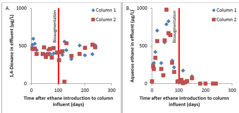
**Figure 5-12.** 1,4-Dioxane and ethane results from the effluent of the duplicate columns (Column 1 and Column 2). The vertical line indicates when the columns were bioaugmented with the MBAFB ethane-oxidizing enrichment culture. Influent 1,4-dioxane and ethane concentrations were prepared at 500 and 700  $\mu\text{g/L}$ , respectively.
