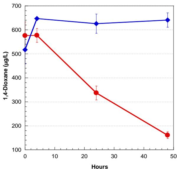
**Figure 5-7.** Biodegradation of 1,4-dioxane by the ethanotroph *Mycobacterium sphagni* ENV482. The blue symbols represent an uninoculated control and the red symbols represent bottles with ENV482. Error bars are form duplicate samples.
