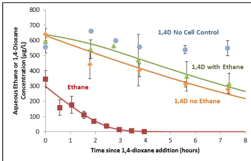
**Figure 5-11.** Coupled biodegradation of ethane and 1,4-dioxane. The solid lines represent the regressed kinetic model. The averages of triplicate samples are shown for 1,4-dioxane, and the averages of duplicate samples are shown for ethane. Error bars represent 95% confidence intervals.
