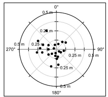
Figure 6-36: Comparison of the Offset Between the Known Location of Blind Seed Items and the Interpreted Target Location (ESTCP, 2009)
