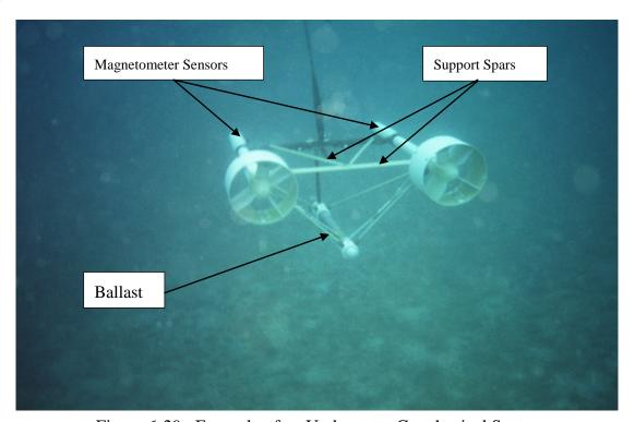
Figure 6-29: Example of an Underwater Geophysical System
