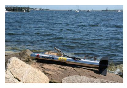
Figure 6-15: Example of an SSS Sensor
