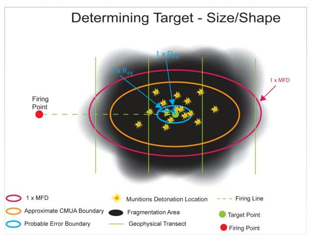
Figure 8-8: Example Determination of Target Area Size and Shape Using the MFD, R<sub>PE</sub>, and D<sub>PE</sub> (Modified from URS Group, Inc, 2009.)
