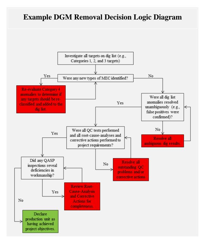
Figure 9-2: Example DGM Removal Decision Logic Diagram
