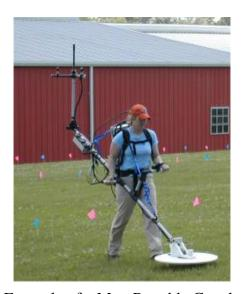
Figure 6-26: Example of a Man-Portable Geophysical System
