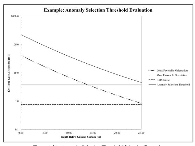
Figure 6-31: Anomaly Selection Threshold Selection Example
