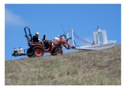
Figure 6-6: Geometrics MetalMapper<sup>™</sup> Advanced EMI Sensor
