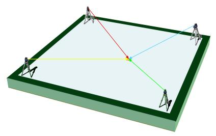
Figure 6-23: Example of a Typical Laser Transmitter Layout
