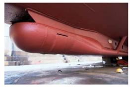
Figure 6-14: Example of an MBES Sensor
