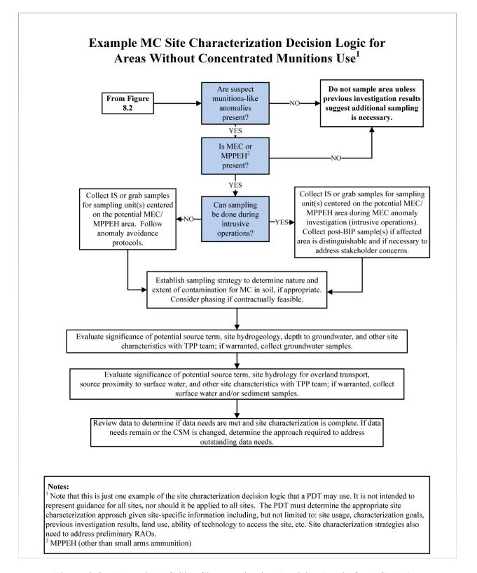
Figure 8-3: Example MC Site Characterization Decision Logic for NCMUAs
