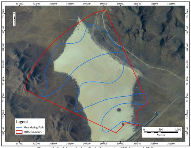
Figure 8-5: Meandering Path Surveying Within an MRS
