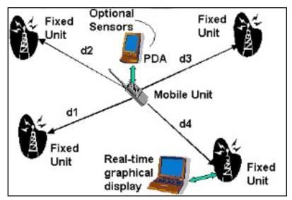
Figure 6-24: Example of an RF Positioning System
