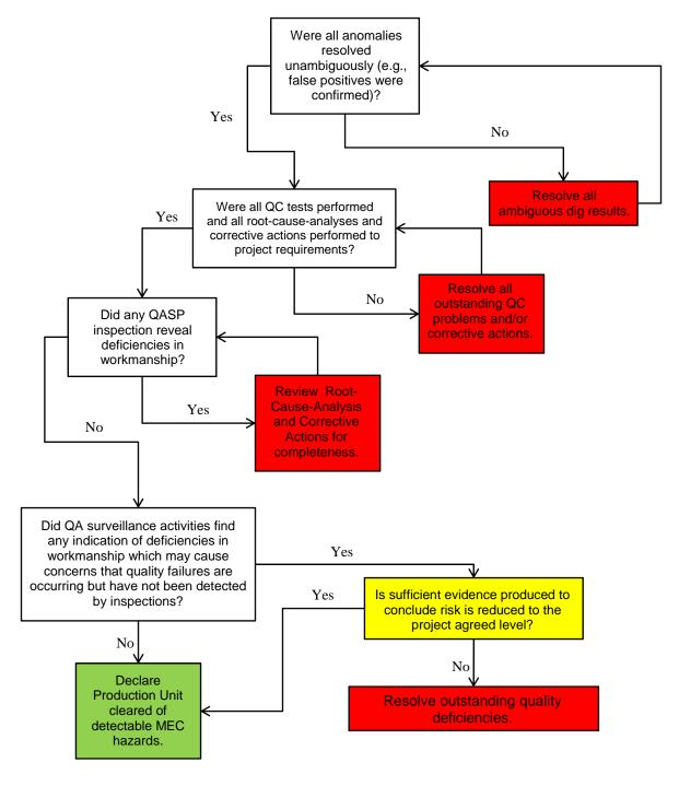
Figure 9-4: Example Analog Geophysical Removal Decision Logic Diagram
