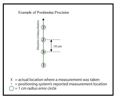
Figure 6-19: Example of Positioning Precision
