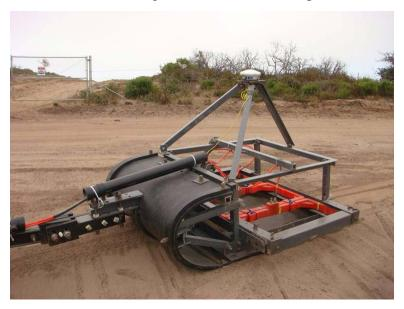
Figure 6-5: Example of a Towed TDEMI Array
