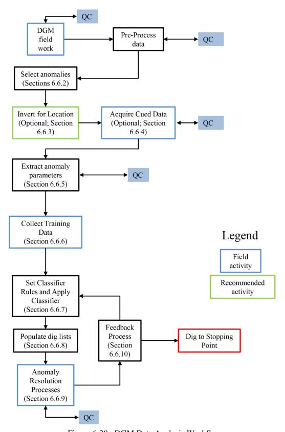
Figure 6-30: DGM Data Analysis Workflow
