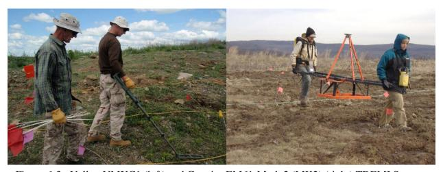
Figure 6-3: Vallon VMXC1 (left) and Geonics EM61-Mark 2 (MK2) (right) TDEMI Sensors
