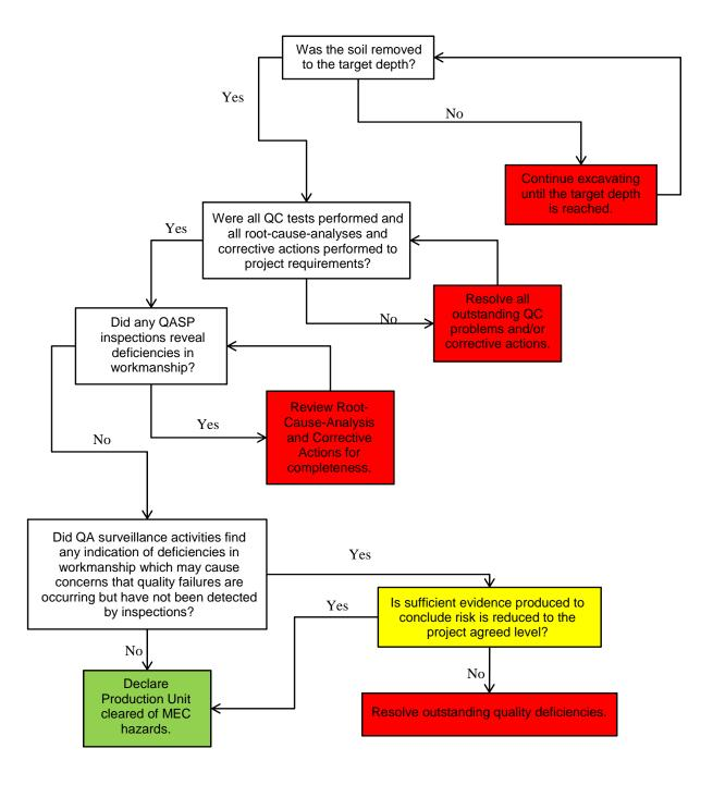
Figure 9-6: Example Mass Excavation Removal Decision Logic Diagram
