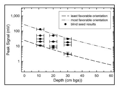
Figure 6-35: Comparison of Blind Seed Response with Their Error Bars to the Theoretical.
