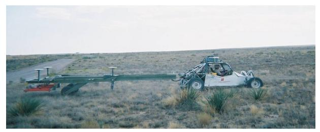
Figure 6-27: Example of a Multiple Instrument Array
