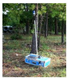
Figure 6-2: Geometrics G-856 Proton Precession Magnetometer
