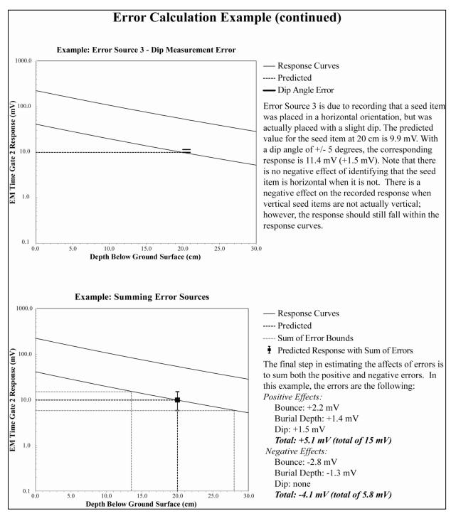
Figure 6-32: Estimating Measurement Variability and Error (continued)
