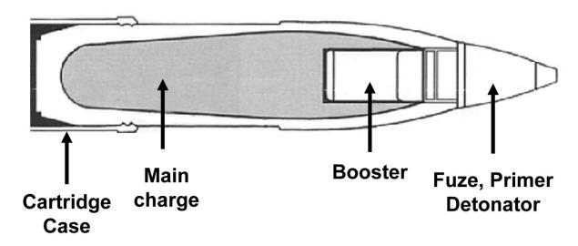
Figure 7-1: Sources of MC in Munitions
