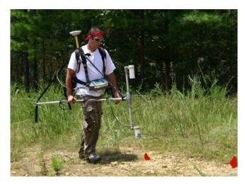
Figure 6-1: Schonstedt GA-52 (left) Fluxgate Magnetometer and Geometrics G-858 (right) Optically Pumped Metal Detector
