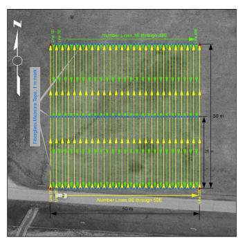
Figure 6-20: Line and Fiducial Grid Setup
