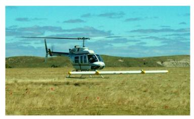
Figure 6-28: Example of an Airborne Geophysical System
