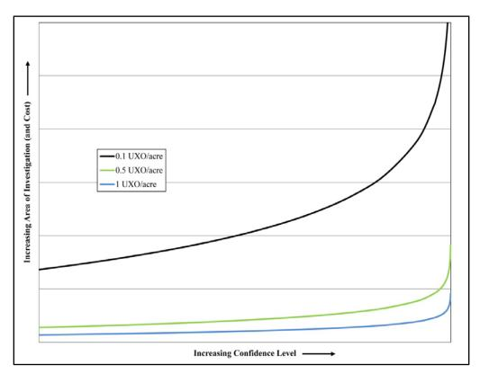
Figure 8-14: Variation of Required Area of Investigation as a Function of Confidence Level for Three Example UXO Densities with a Constant Site Size.
