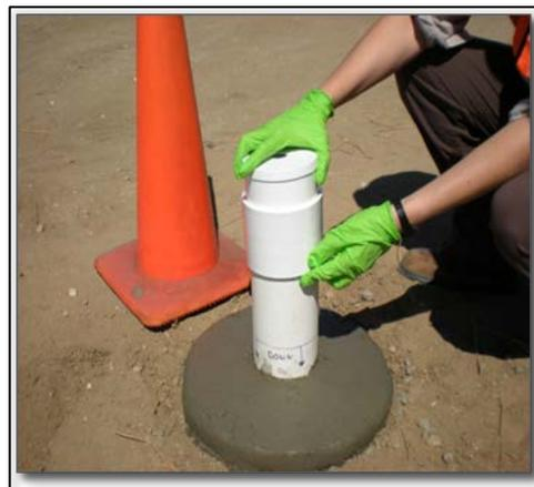
CO<sub>2</sub> trap developed by Colorado State University to measure LNAPL loss rates in the field <sup>121</sup>
