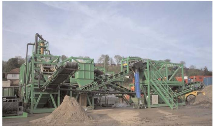
Fig.1: Mobile soil washing plant (Courtesy of DEC NV)
