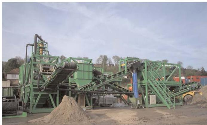
Fig.1: Mobile soil washing plant (Courtesy of DEC NV)
