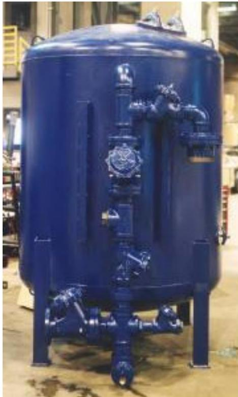
Figure 7-7. Pressurized Media Filter (U.S. Filter).
