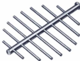
Figure 7-5. Header-Lateral Distribution System (Johnson Screens).
