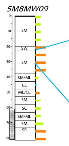
This SM interval is a fine to coarse grained Silty Sand with gravel, representative of a channel deposit.
