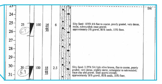
Both were logged as SM, but the details show that they have significantly different depositional characteristics.
