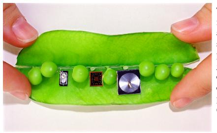
Three principal components of Sandia's integrated micro chem lab are small enough to fit easily inside a snow-pea pod. Shown from left to right are a surface acoustic wave sensor array, a preconcentrator that collects chemical vapors for gas-phase analysis and a miniature gas chromatograph column. The entire system, designed to also analyze liquid samples, fits into a package about the size of a thick paperback book. (Photo by Randy Montoya)
