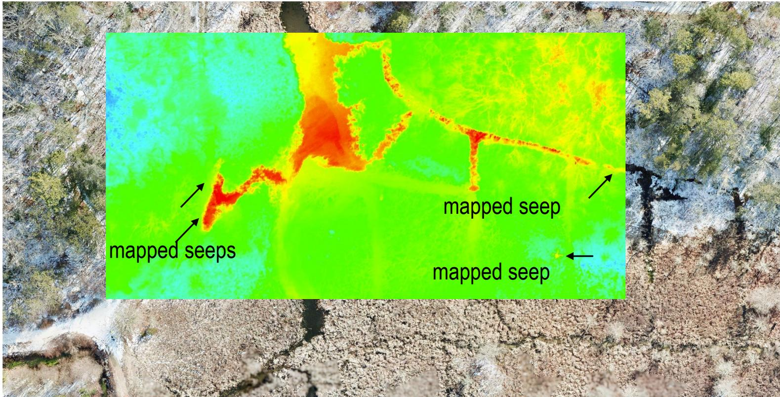
Thermal IR data overlaid on the RGB base map shows how several seeps that were located by handheld thermal IR were also evident in the drone-based data, and major discharge accumulation zones along the larger channel features were also noted.
