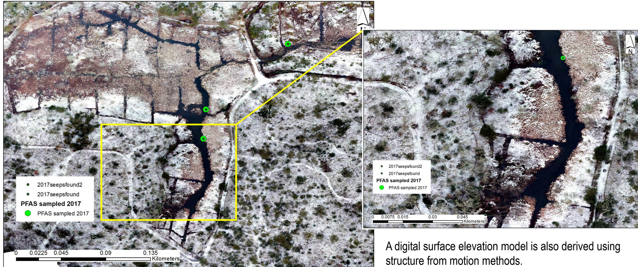
A digital surface elevation model is also derived using structure from motion methods.
