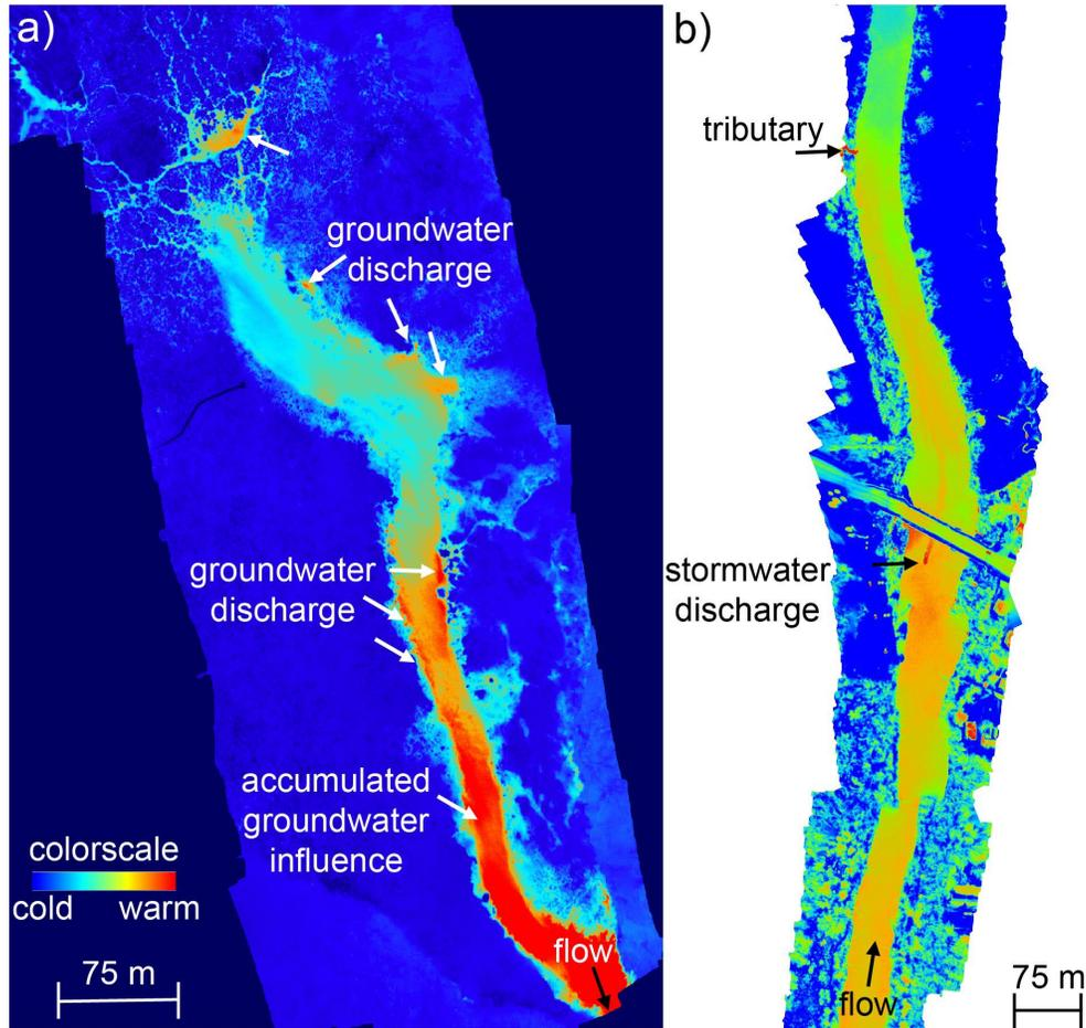
UAS-based thermal IR can efficiently map large areas under favorable conditions
