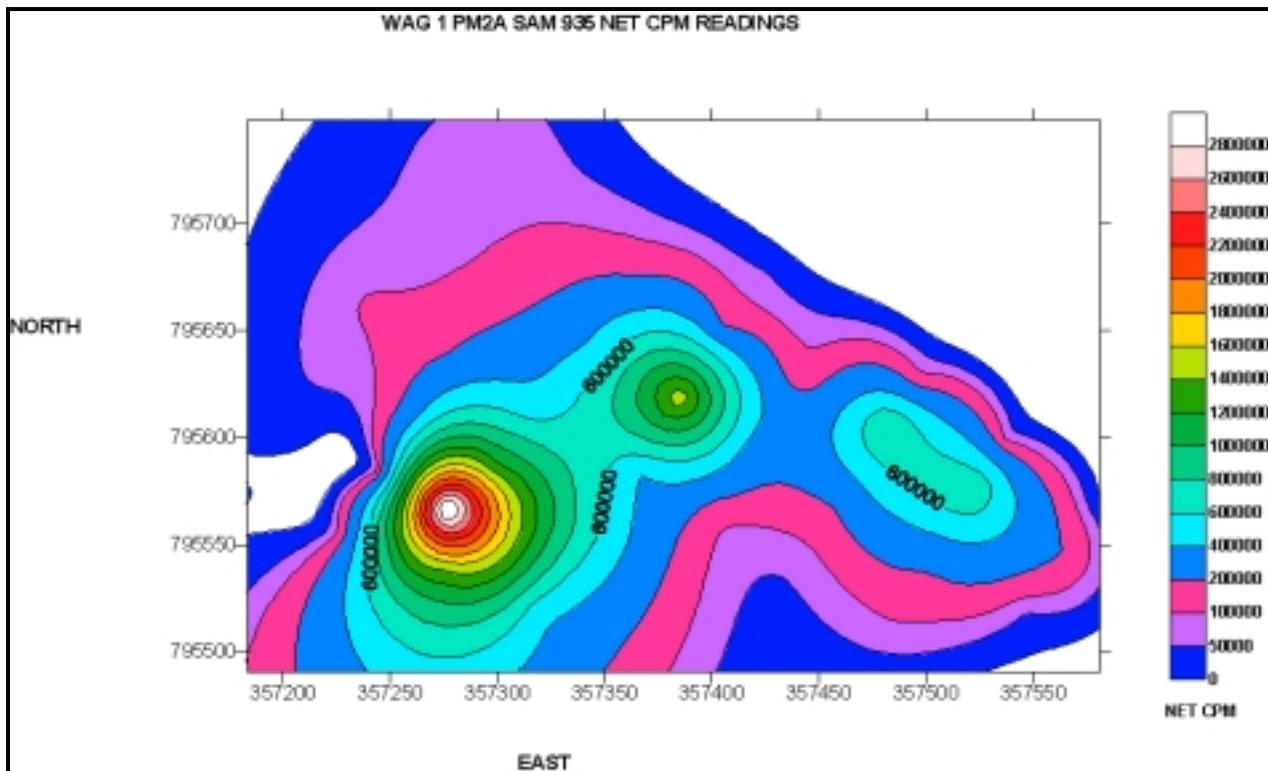
Figure 6. PM-2A radiation map generated from SAMS readings.
